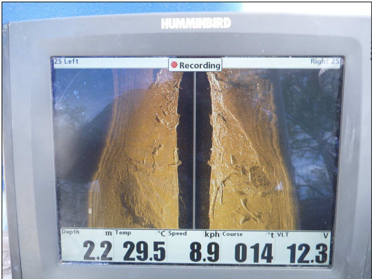
Figure 7. Side-scanning sonar recording instream habitat features.
